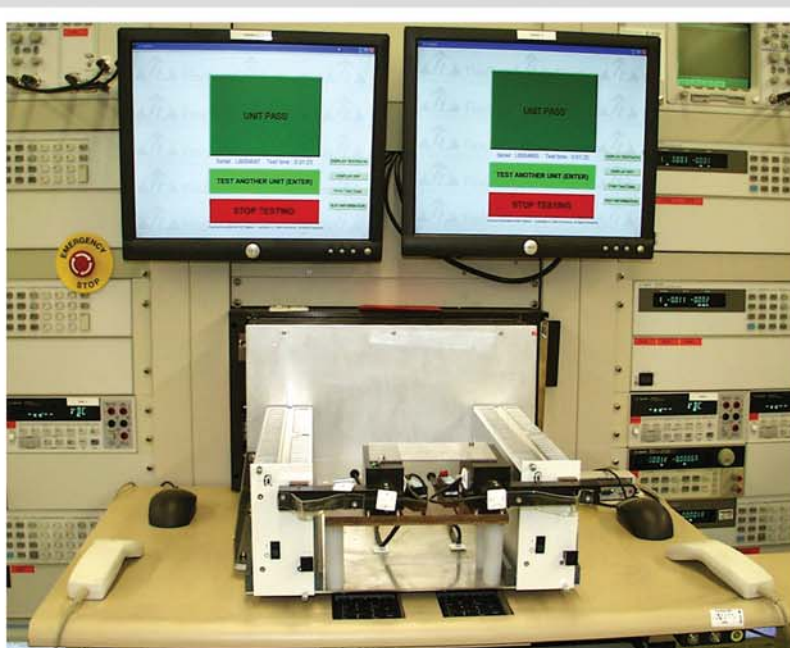
Two UUTs in a dual Test Fixture
