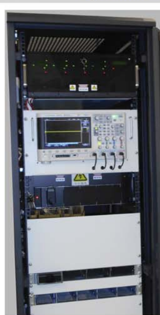
Fixture with added HV Loads and Scope
