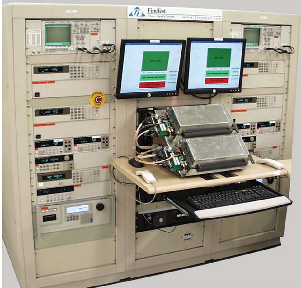
Dual Tester with two UUTs installed in the Test Fixture
